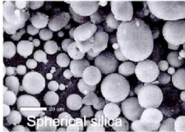
Figure 2- Higher magnification images of silica flakes (left) and spherical silica (right).
