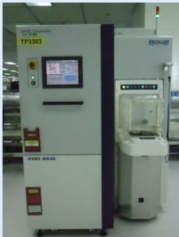
Taper system and loading system
