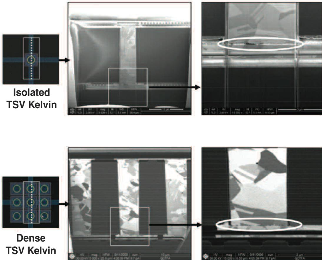
Another TSV failure mechanism is copper extrusion. This can happen when the compressive stress on the copper causes the copper to extrude into the surrounding layers. This can lead to a short. The image above shows an example of extrusions occurring on both sides of the TSV.
