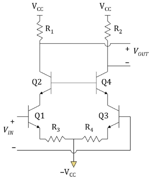
Let's look at a different, and more popular, way to implement the Class A amplifier. This slide shows an example of a Class A common base output stage. In this example the output voltage is the difference between the voltages on the collectors of Q2 and Q4. This is controlled by the input voltage, which is the difference between the voltages on the bases of Q1 and Q3. Although we show bipolar circuits in these figures, designers can implement Class A amplifiers in both bipolar and CMOS.
