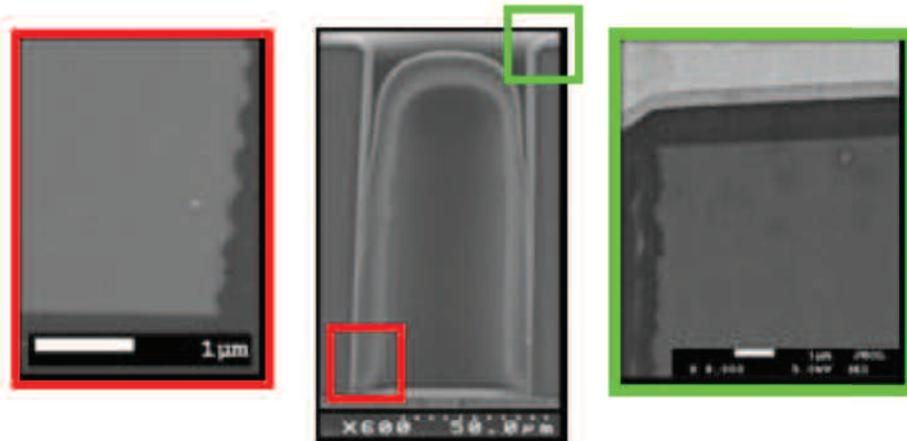
Yet another TSV failure mechanism is voiding. This can occur at the interface between the copper TSV and the metal layers. The voiding leads to increased resistance in the via, and the possibility of
