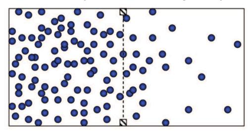
occurs, even at very low temperatures. Not only does this occur in semiconductor materials, but it is also associated with other mechanisms, like intermetallic growth. For instance, Kirkendall voiding with intermetallic growth as an example of this, since diffusion of gold into aluminum occurs more quickly than diffusion of aluminum into gold.
