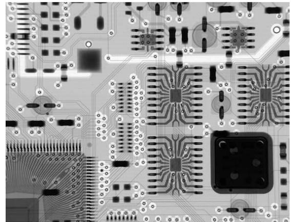
Figure 1. Top: Digital x-ray radiography image
