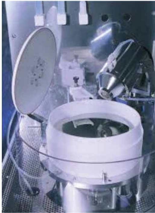
Figure 1. Ozonated De-ionized Water Cleaning System.
