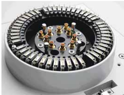
Figure 3. Illustration of 4083A test head direct docking scheme .
