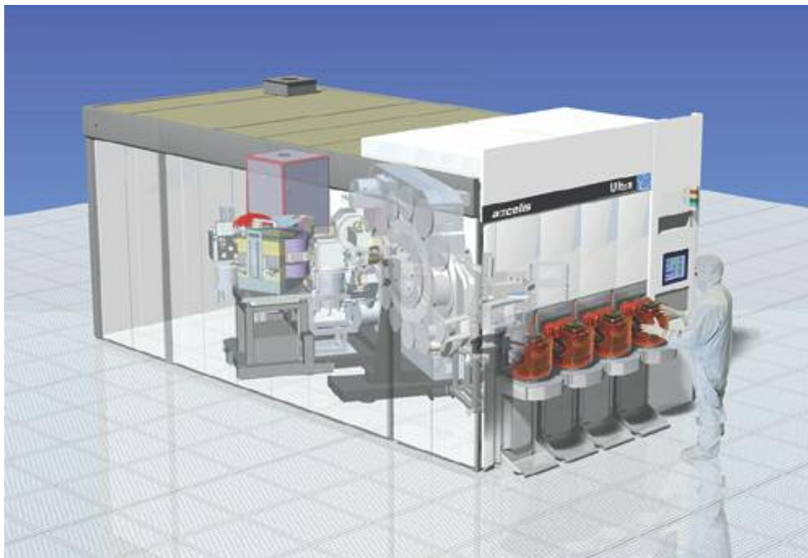
Figure 1. Model of a typical high current implanter (image courtesy Axcelis).
