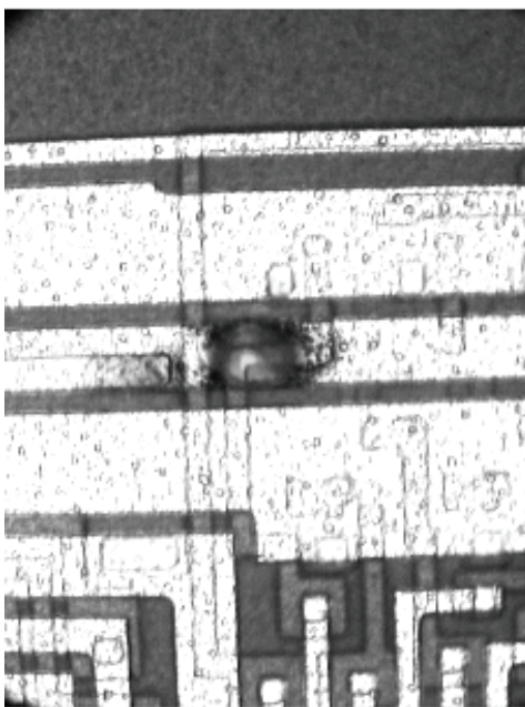
Figure 6. Example of a customer return failing from Electrical Overstress (EOS).
