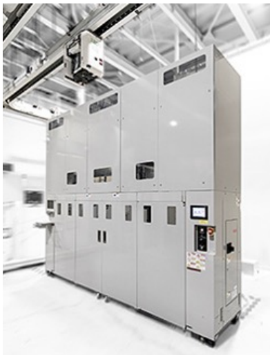
Figure 5- Tool Front FOUP Buffer. Image courtesy Murata Machinery, Ltd.
