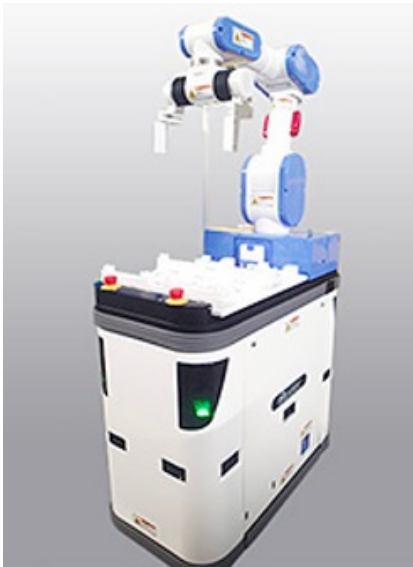
Figure 3- Automated Guided Vehicle (AGV). Image courtesy Murata Machinery, Ltd.
