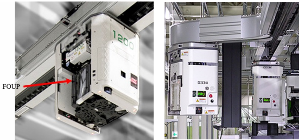
Figure 1- (Left) Overhead Transport (OHT) with FOUP, and (Right) portion of Overhead Transport system with two OHT units visible. Images courtesy Murata Machinery, Ltd.
