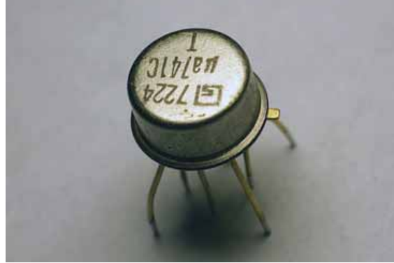
Figure 3. Example of uA741 op amp.
