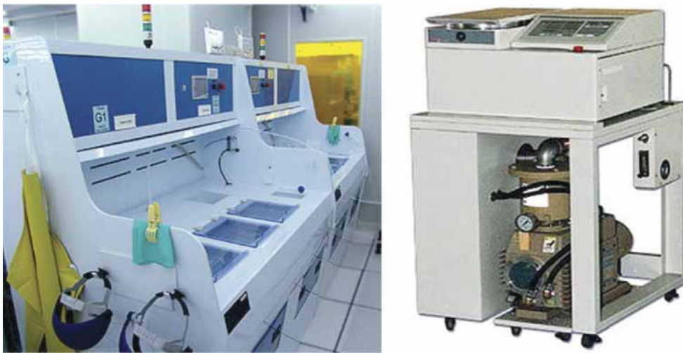
Figure 4. Chemical Etch System for Wafer Thinning (left) and Plasma Etch System for Wafer Thinning (right).
