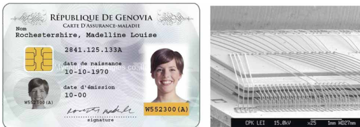
Figure 1. Smart Card (left) and Stacked Die Structure (right).
