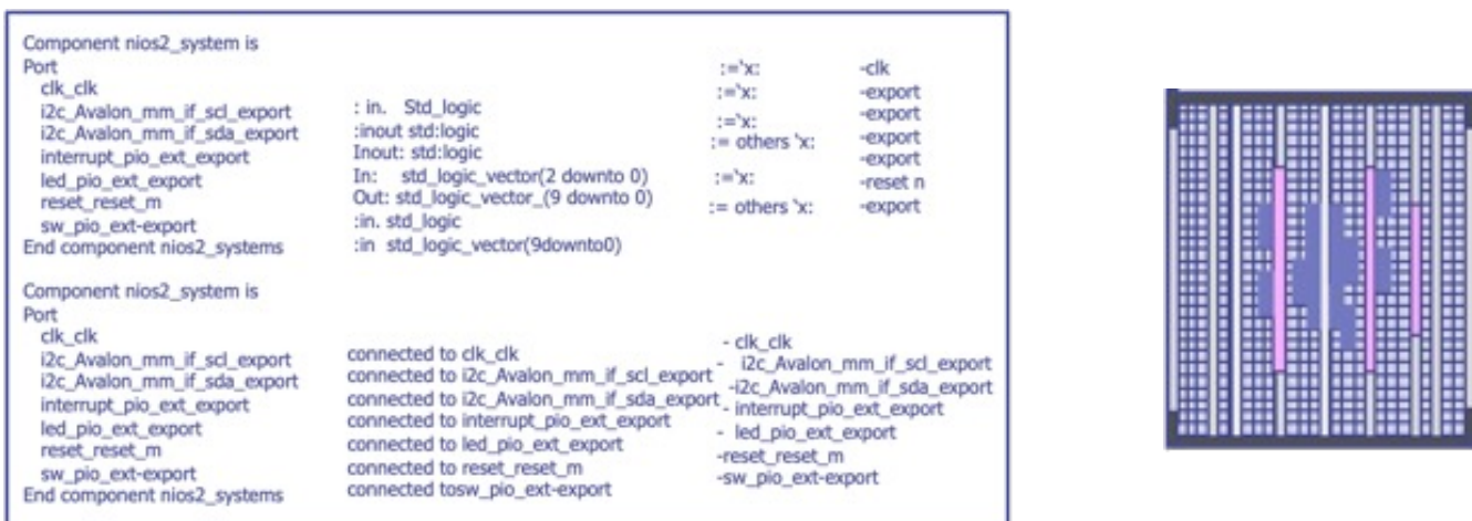
Figure 1- An excerpt from the VHDL code of a Soft Core processor (left), and the physical implementation of the Soft Core processor (right)
