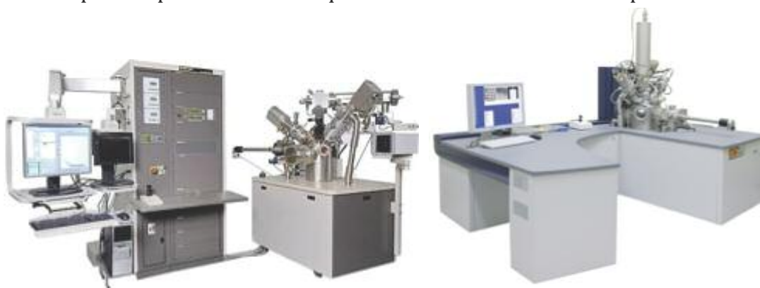
Figure 1. Secondary Ion Mass Spectroscopy Equipment (left: Quadrupole SIMS; right: Time of Flight SIMS). Images courtesy Cameca and Ion-TOF
