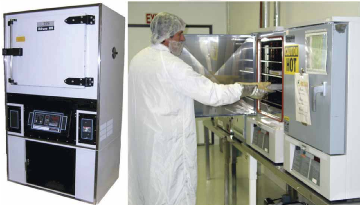
Figure 6. Equipment for die attach curing process.
