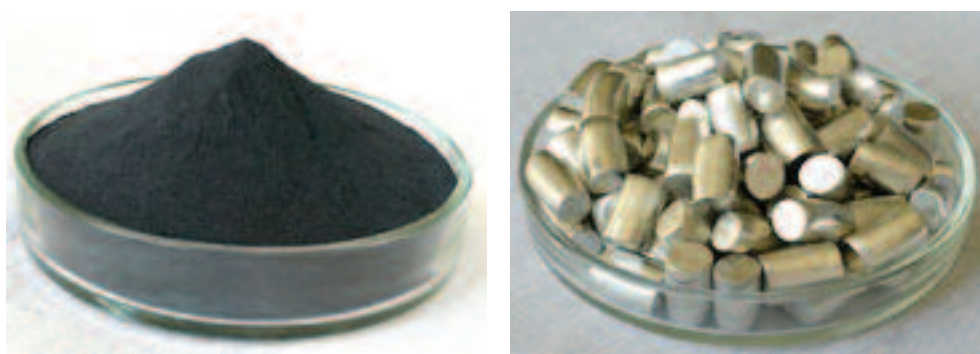
Figure 2. Low alpha tin oxide powder (left), and low alpha tin pellets (right)
