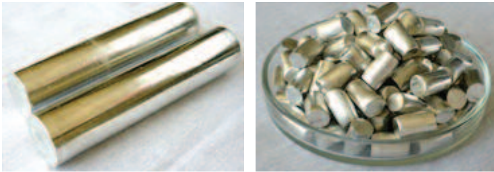
Figure 3. Low alpha lead - 4N purity (left), and low alpha lead pellets (right)
