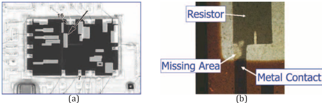
Figure 1. (a) Resistor network chip used inside a hybrid microcircuit, and (b) Portion of a nichrome thin film showing a missing area of the element.
