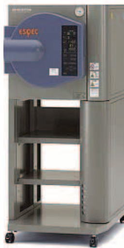
Figure 7. Illustration of specialized oven for HAST testing from ESPEC.
