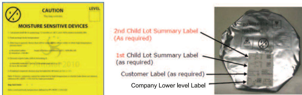
Figure 2. Moisture sensitive devices label (left) and dry pack shipping bag (right).
