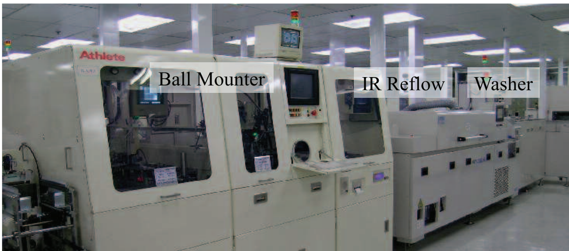
Figure 3. Ball attach reflow and wash equipment.
